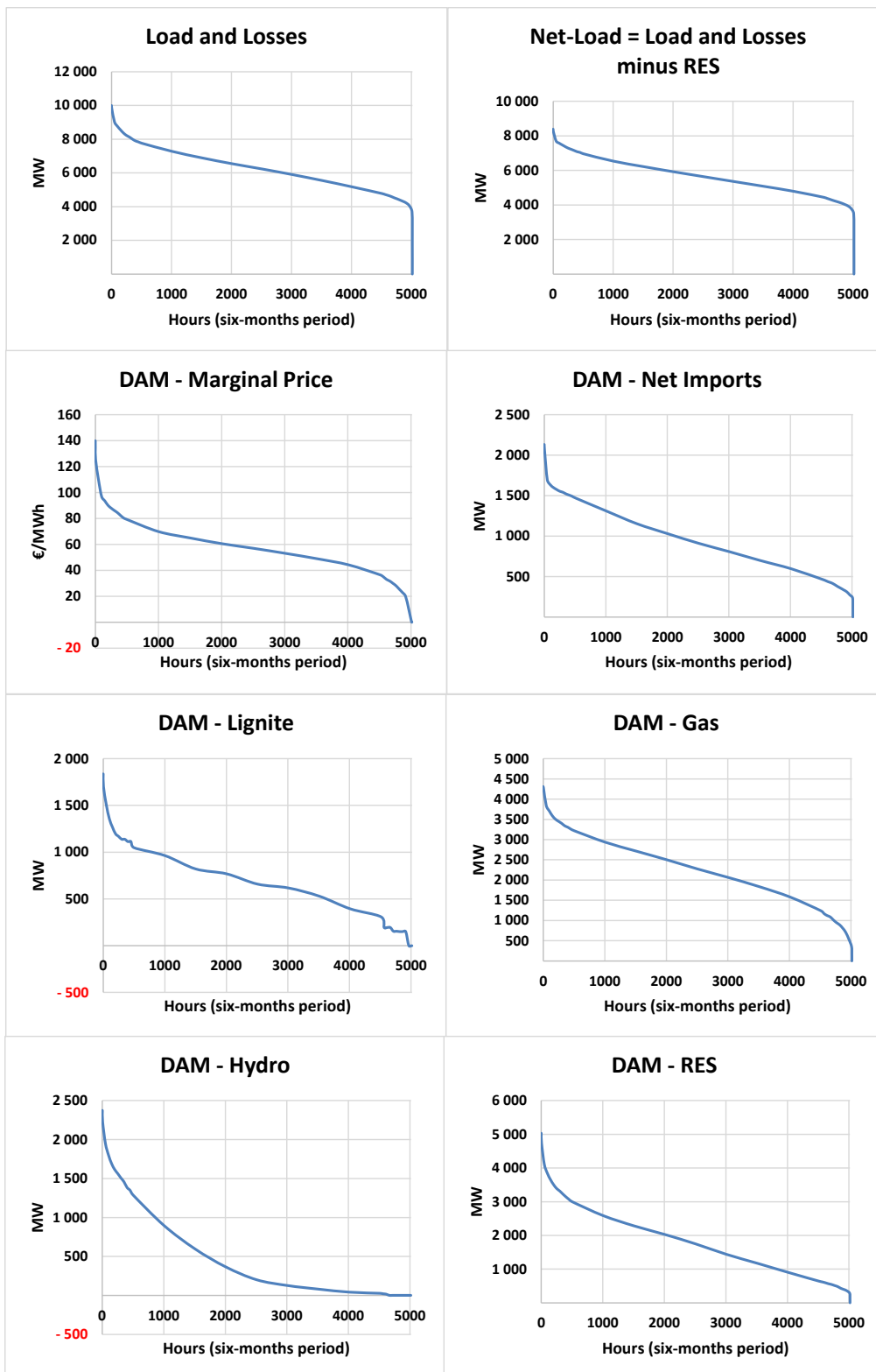
Figure 8: Duration curves for load, marginal market prices and generation schedule, according to the DAM
